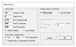
A separate form has also been made for hole milling, where the different options for hole milling can be easily specified. A new adjustment option is to enter the entry angle instead of the cutting depth in ramp machining. Now, you can also choose between climb-cut and up-cut milling.
