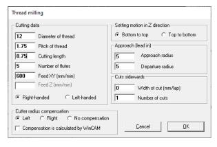
The most requested development by users has been the diversification of thread milling. In the new version, it is now possible to cut either inwards or outwards in Z-direction. Multiple side cuts have also been added. All in all, defining thread milling in the new form is much easier than before; even the diameter and pitch of the thread can still be adjusted during the programming phase - as well as the threading length or number of teeth of the thread mill.
