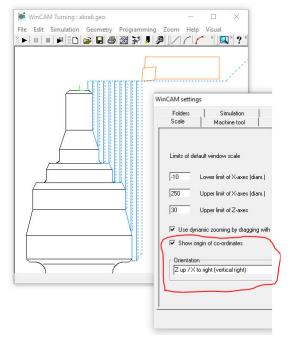
In version 3.2.0, the long-desired reform for vertical lathes was implemented. Now, when simulating turning and defining the geometry, the position of the coordinate system (workpiece) can be chosen so that it looks the same as it does at the lathe. The workpiece can now be upright on the table, and the tool can approach from either the right or the left. With a horizontal lathe, the tool can approach from above or below.
