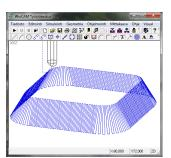
As a new machining method, the axial milling option of path milling has been added with the possibility of machining in a zigzag manner so that the lateral movement takes place alternately at the top and bottom, i.e., the tool is cutting all the time. This machining method is often not successful in roughing, but in finishing, it speeds up machining and improves the surface quality. Zigzag-type axial milling can be used both for vertical and inclined profiles.
