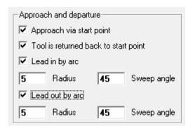
The option to approach and exit with an arc movement has been added to the finishing function of turning. Arc radius and sweep angle can be set.
