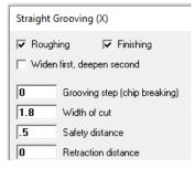
In addition to the safety distance, a separate retraction distance has been added to all the grooving and cutting functions of turning, which enables grooving operations without the risk of collision to the bottom of a cavity - e.g., another groove.
